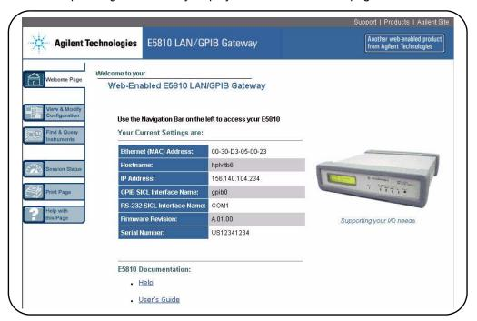
You can use the Web access to configure the E5810 and to communicate with GPIB and/or RS-232 instruments. For example, using the **Configuring your E5810 LAN/GPIB Gateway** page of the E5810 interface, you can view and modify the configuration of the E5810. Or, you can communicate with installed GPIB and/or RS-232 instruments using the **Find and Control Instruments Connected to your E5810** page of the interface. See *Chapter 3 - Using E5810 Web Access* for information on E5810 Web access.
