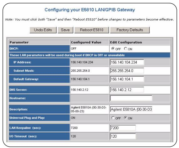
4 Set E5810 for Enterprise Network Operation. To properly set E5810 configuration parameters for eventual use on an Enterprise network, you may need to enter the following network values, as provided to you by your System Administrator, on the Configuring your E5810 LAN/GPIB Gateway page
